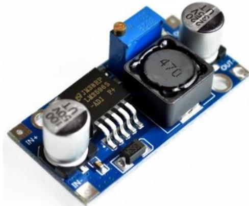
Figura 31. Conversor DC a DC ajustable
